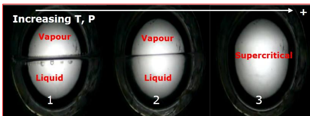
Fig. 1.2: Phase boundary of fluid with temperature and pressure adapted [8].
